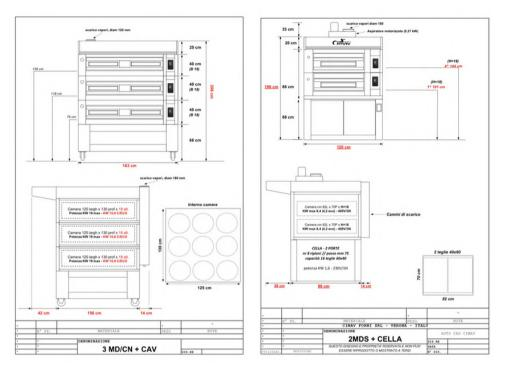
The technical data sheets, attached to the offers, allow you to fully understand the dimensions of the oven, the electrical power and all aspects related to hydraulic, electrical and flue connections.
